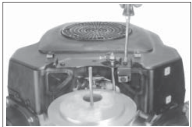
Figure 11-75. Installing Control Panel.
